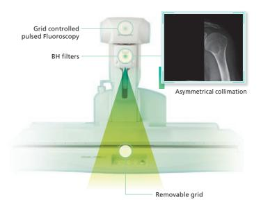
Asymmetrical collimation, on either the left or right can be applied, eliminating exposure outside the ROI.
