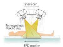
Imaging technology that fuses cone-beam CT reconstruction with digital image processing.
