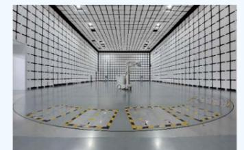
Quality Center's 10-Meter Method Anechoic Chamber
