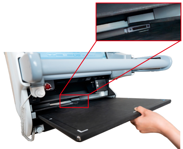
Fig.3 FPD Docking Mechanism
