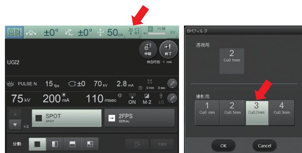
Fig.11 Accessory Filter Thickness Adjustment Windows
