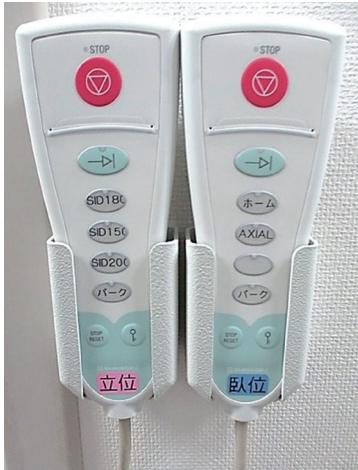
Fig.4 Remote Controllers for Automatic Positioning for Radiography in Standing and Supine Positions Controller for Standing Position (Left) • SID150: Lateral view of thoracic vertebrae, lateral view of lumbar vertebrae, etc. • SID180: Chest, cervical vertebrae, etc. • SID200: Auto-stitching radiography • Park: X-ray tube position when not in use Controller for Supine Position (Right) • Home: Anterior view of lumbar vertebrae, etc. • AXIAL: Axial position of patella, etc. • Park: X-Ray tube position when not in use
