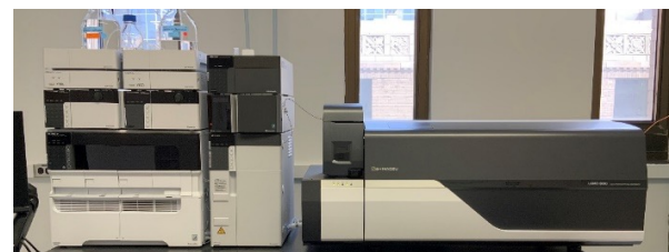
LCMS-8060 High-Performance Liquid Chromatograph Mass Spectrometer System Used for Joint Research with Washington University
