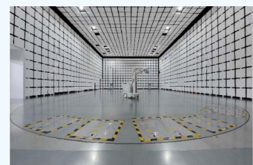
Quality Center’s 10-Meter Method Anechoic Chamber
